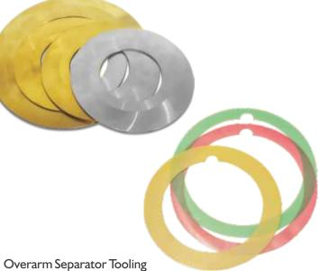
**Separator Discs-** The discs are subject to heavy wear & impact, hence the raw material should be wear & shock resistant. Also they should not be so hard that they damage coils edges. Most common grades are CrV Alloy Steel, 100Cr6, SAE4340/EN24, 1.2379/D2. The separator discs can be supplied with TiN coating or chrome plating to improve their wear resistance. Generally hardness of 52/56 HRc works well.
