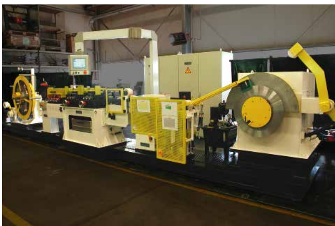
DUO strip edge trimming line with decoiler, flat levelling machine, vertical levelling machine, DUO strip edge trimming machine, strip width measurement, strip tension regulation, S-bridel and dancer and recoiler
