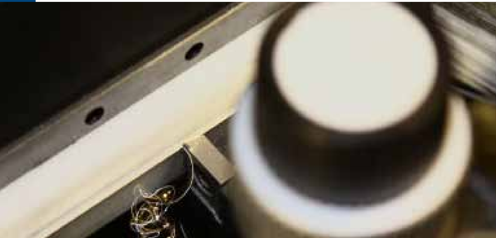
Onesided edge machining of an aluminium strip
