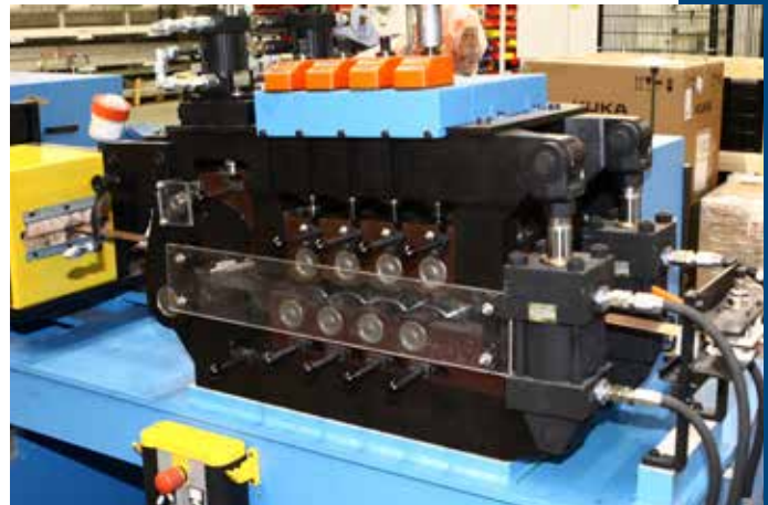
Flat levelling machine type DR61 with alligator system
