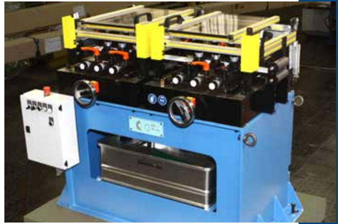
The strip edge trimming machine of the series DUO works with 6 tools. Often the DUO is integrated into tube production lines to optimize the weld seam.
