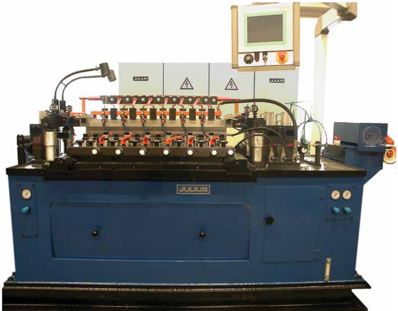
Strip edge trimming machine of the series BKB-compact with six (seven) tools
