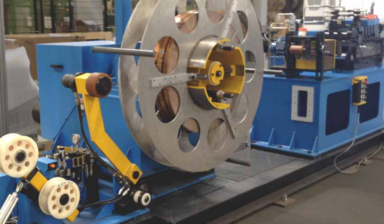
CNC controlled strip edge trimming and oil grooving line with multicoil system
