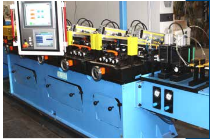
The QUINTO strip edge trimming machine works with up to 15 tools and achieves each contour required.
