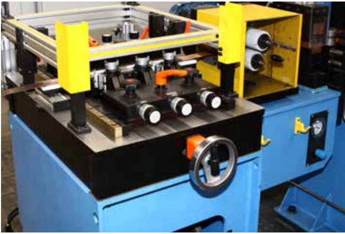
The strip edge trimming machine of the series UNO works with one tool each side. It is the smallest machine of the modular system being employed for simple deburring of the strip edge.
