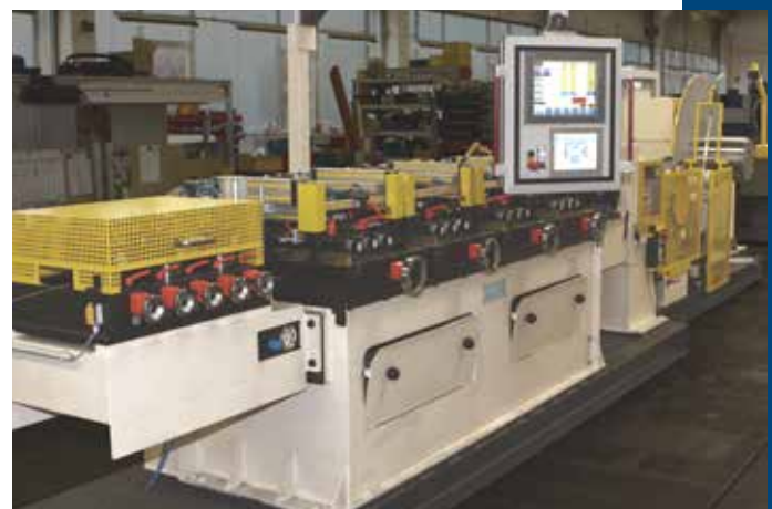
Strip edge trimming line with vertical levelling machine, QUATTRO strip edge trimming machine, strip width measurement, strip tension system with S-bridel and dancer as well as recoiler and turnstile (not on the picture: aperture roller and flat levelling machine)
