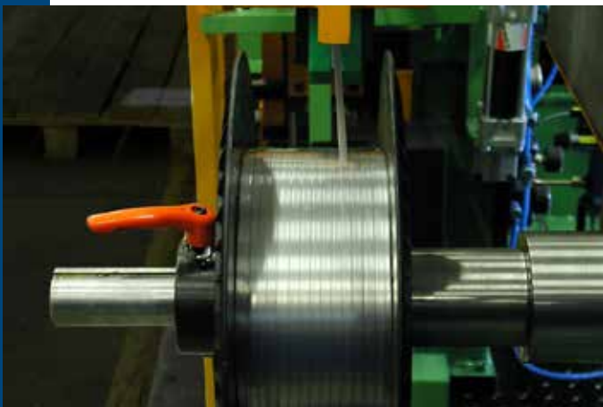
Traverse rewinding of small strips with cassette and flanged adapter
