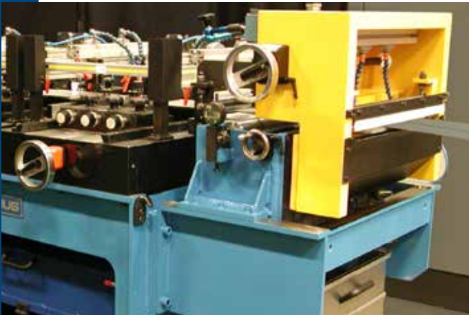
Grooving machine of the series NU with one tool – here flanged at a TRI-NU strip edge trimming machine
