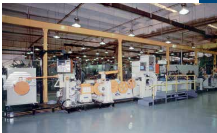
CNC controlled strip edge trimming and oil grooving line for the production of plain bearing bushes and half bearing shells
