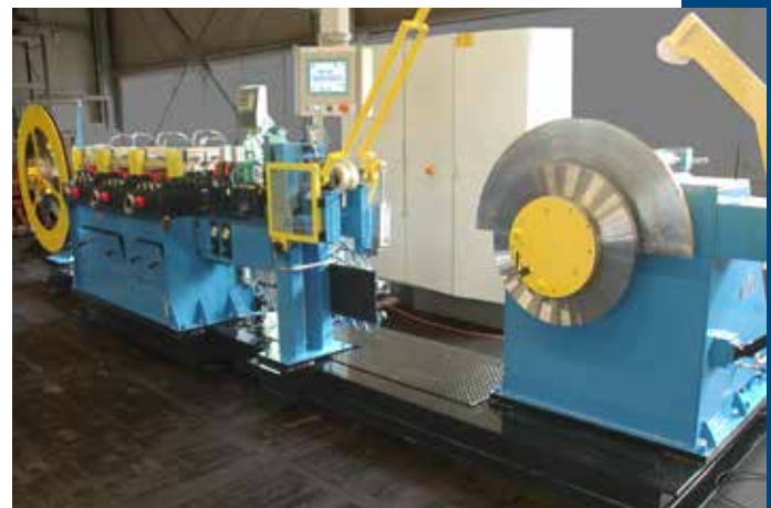
Basic line with decoiler, TRIO strip edge trimming machine, strip width measurement and recoiler
