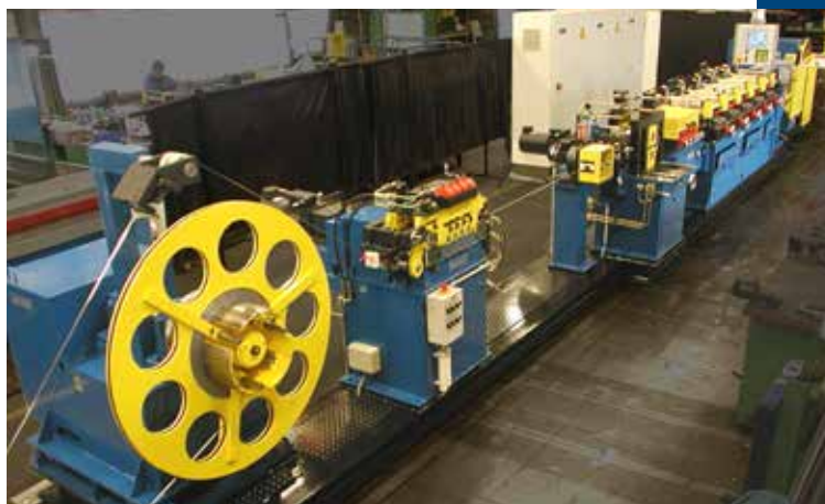
Strip edge trimming line of the series QUINTO for the production of saw bands
