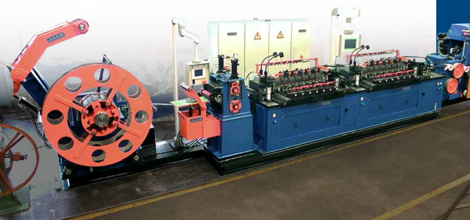
Strip edge trimming line of the series BKB-double-compact with (from left to right): multicoil, decoiler, strip entering system, two compact strip edge trimming machines with six (seven) tools each, S-bridel and dancer for strip tension reduction and recoiler (not on the picture)
