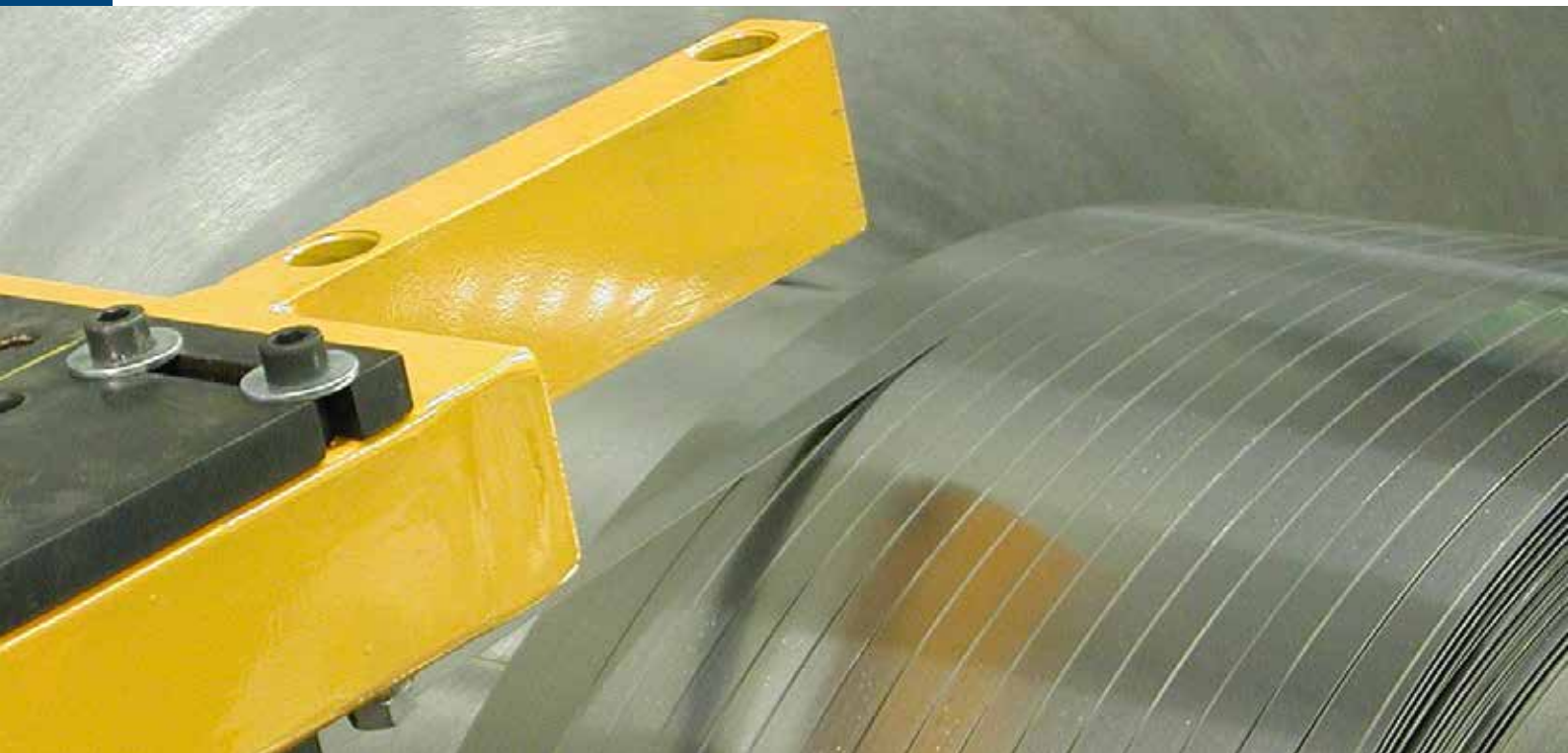
Traverse winding at the recoiler side: Due to a fixed spool guide a high exactitude of traversing is achieved. Picture on the right side: S-bridel, dancer and recoiler
