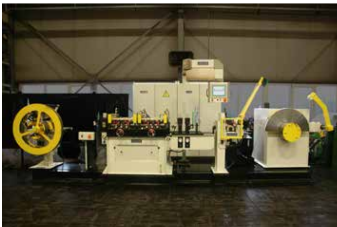
Basic line with decoiler, DUO strip edge trimming machine and recoiler
