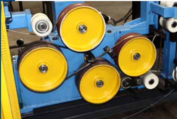
Extended S-bridel for the treatment of teflon coated strips
