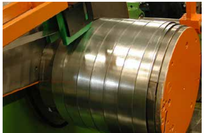
Traverse rewinding of wide strips
